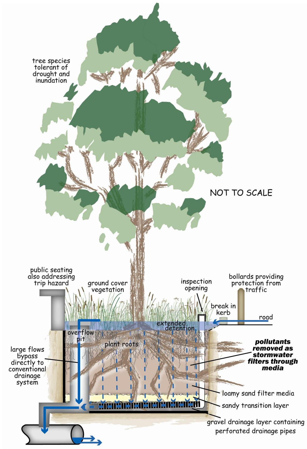
Figure 1. Concept illustration of a raingarden or bioretention tree pit illustrating stormwater flow pathways and subsurface infrastructure requiring maintenance
