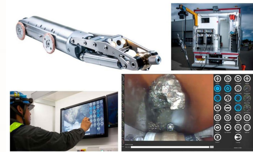
Figure 9.2 Ultra-high-pressure jetting tool with truck and operator controls. Source: vandervalk+degroot BV.
